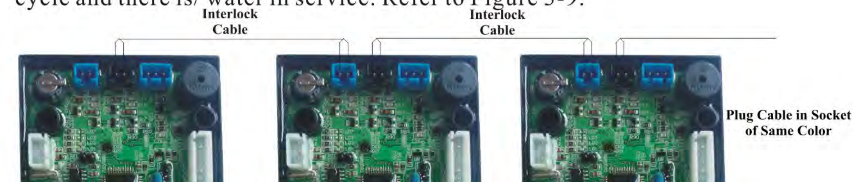
Figure 3-9 Network System Wiring with Interlock Cable
