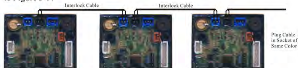
Figure 3-9 Network System Wiring with Interlock Cable
