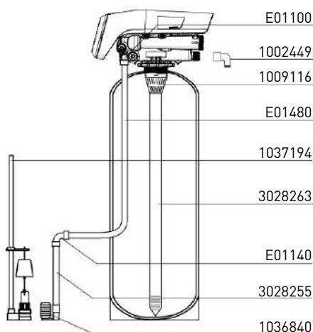
Correct drain line flow control must be fitted depending on media type and vessel size.
