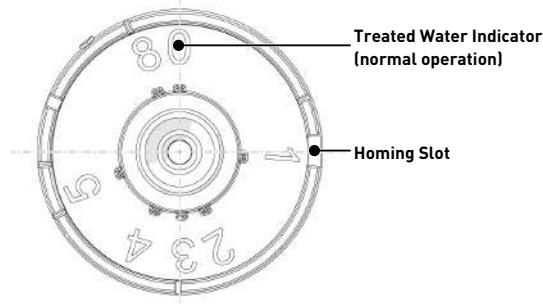
The corresponding slot for the number is positioned at the optical sensor which is approximately 90 degrees out of phase.
